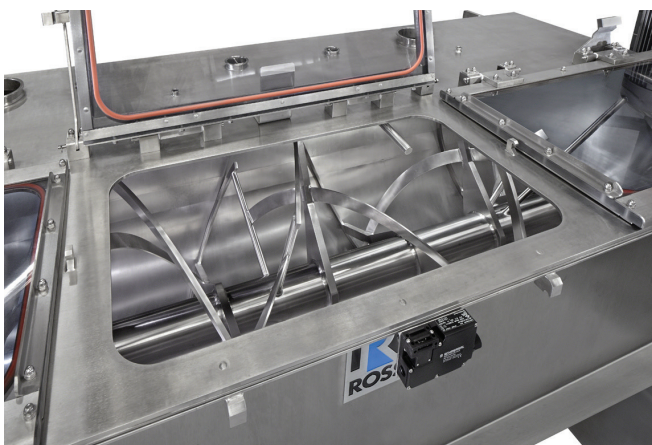
A typical ribbon blender has a U-shaped trough and an agitator made up of inner and outer helical ribbons
